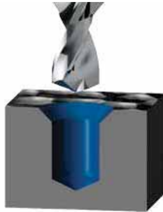
Pilot Hole Drilling
