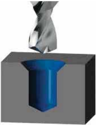
Pilot Hole Drilling
